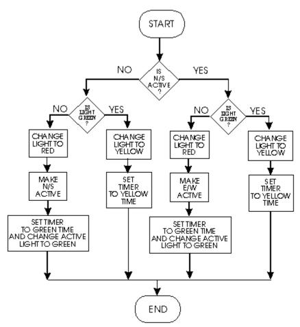
Notice that the two sides of the flow chart are exactly the same with the exception of the line that makes one side or the other the active side.
